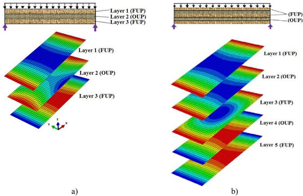
**Fig. 2.** Normal stresses distribution  $\sigma_x$  median surface of each layer of material (FUP - layer reinforced with natural fibres, OUP - layer reinforced with oak particles)
