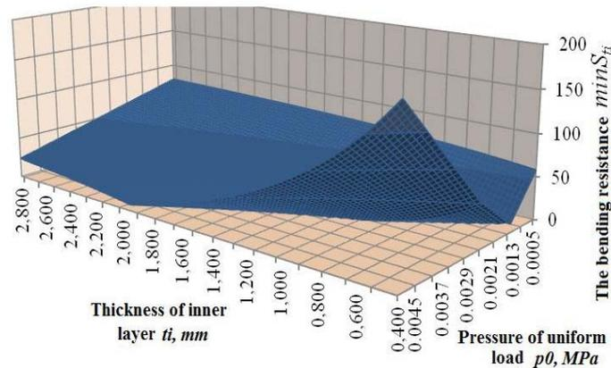
Fig. 10. Variation of  $minS_{ti}$  depending on the thickness of the core and the pressure applied to the plate
