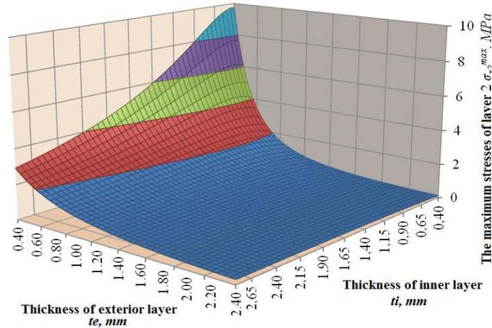
Fig. 7. Variation of maximum stresses in the core layer depending on the thicknesses of layers
