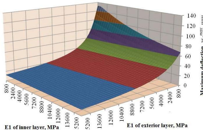
**Fig. 8.** Variation of maximum deflection depending on the longitudinal modulus
