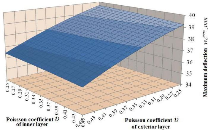
Fig. 9. Variation of maximum deflection depending on Poisson's coefficient
