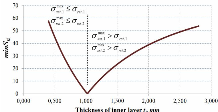
**Fig. 11.** Variation of flexural strength  $\min S$  versus thickness of inner layer
