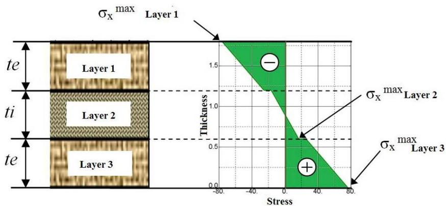
**Fig. 3.** Normal stresses distribution  $\sigma_x$  on composite thickness
