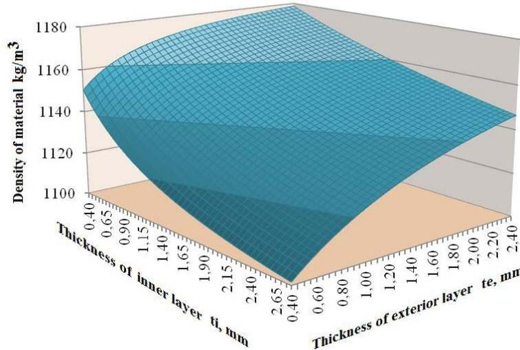
Fig. 4. Variation of density composite depending on the thickness of layers ( $t_i, t_e$ )
