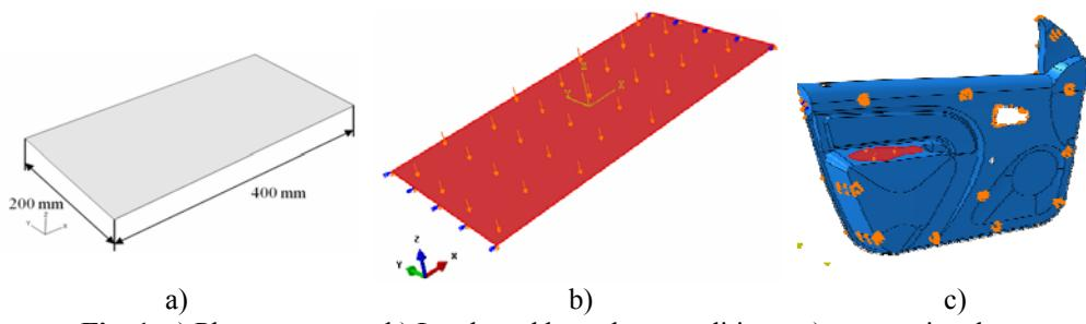
**Fig. 1.** a) Plate geometry; b) Loads and boundary conditions; c) automotive door
