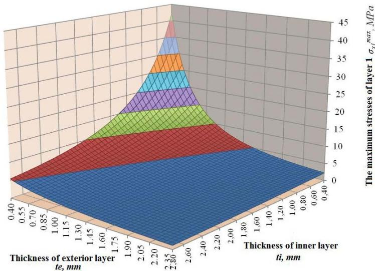
**Fig. 6.** Variation of maximum stresses in the outer layers depending on the thickness of layers
