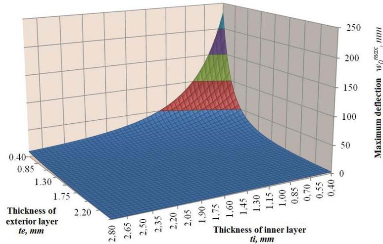
**Fig. 5.** Variation of maximum deflection with thickness of layers
