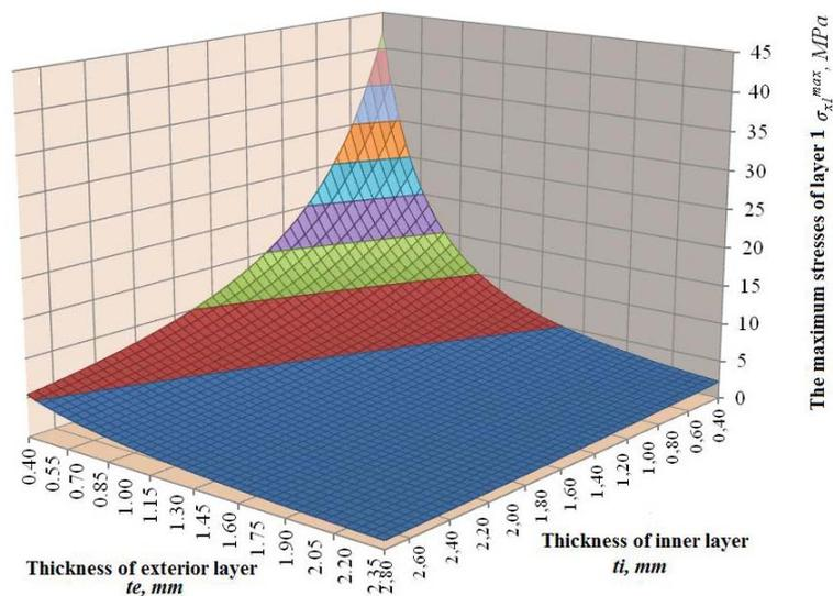
**Fig. 6.** Variation of maximum stresses in the outer layers depending on the thickness of layers
