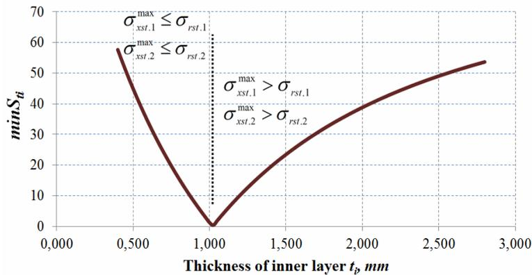
Fig. 11. Variation of flexural strength  $minS_{fl}$  versus thickness of inner layer
